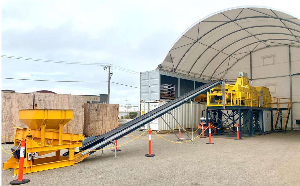
Figure 1: Full scale Steinert KSS ore sorter, Bibra Lake, Western Australia
