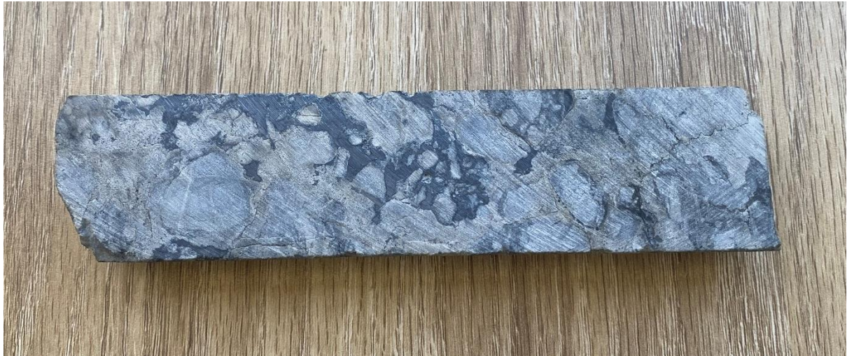
Figure 2: Drill core from STOR1601D from interval 97-101m downhole – average grade 4.16%. The Chalcocite is seen as the dark gunmetal grey material within the lighter grey dolomite host rock.
