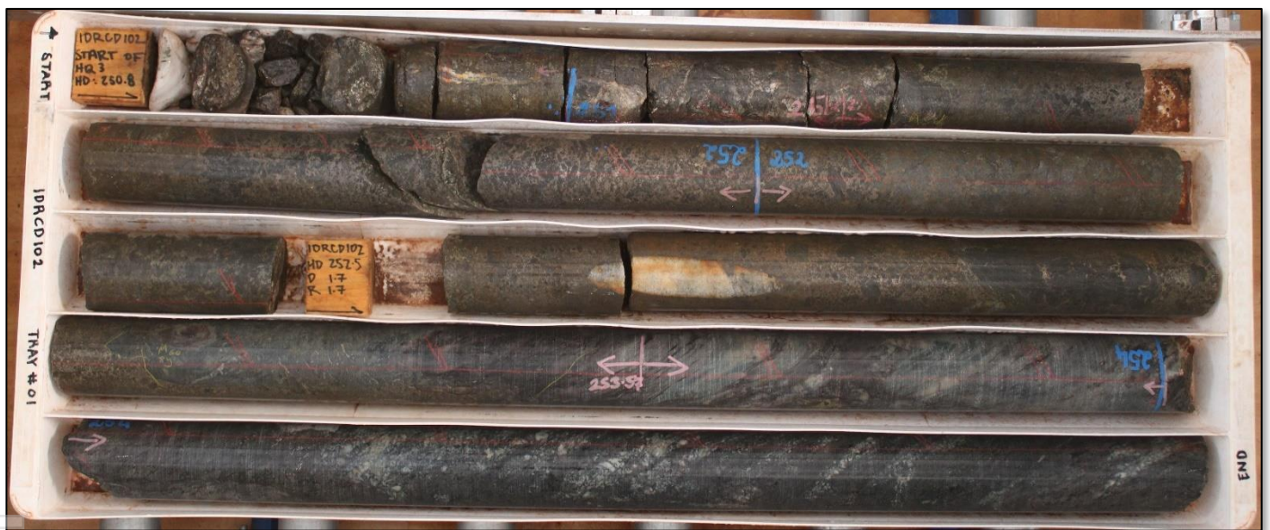
Figure 11; IDRCD102 HQ drill core intersected massive to semi massive sulphides predominantly pyrrhotite, pyrite with minor Chalcopyrite from 250.8 to 253.7m #
