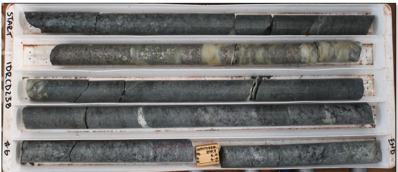
Figure 9; IDRC238; Uncut diamond showing 1.2m of semi-massive sulphide (Pyrrhotite and Chalcopyrite) in quartz veining within and Anorthosite country rock (206.9m to 208.3m) #
