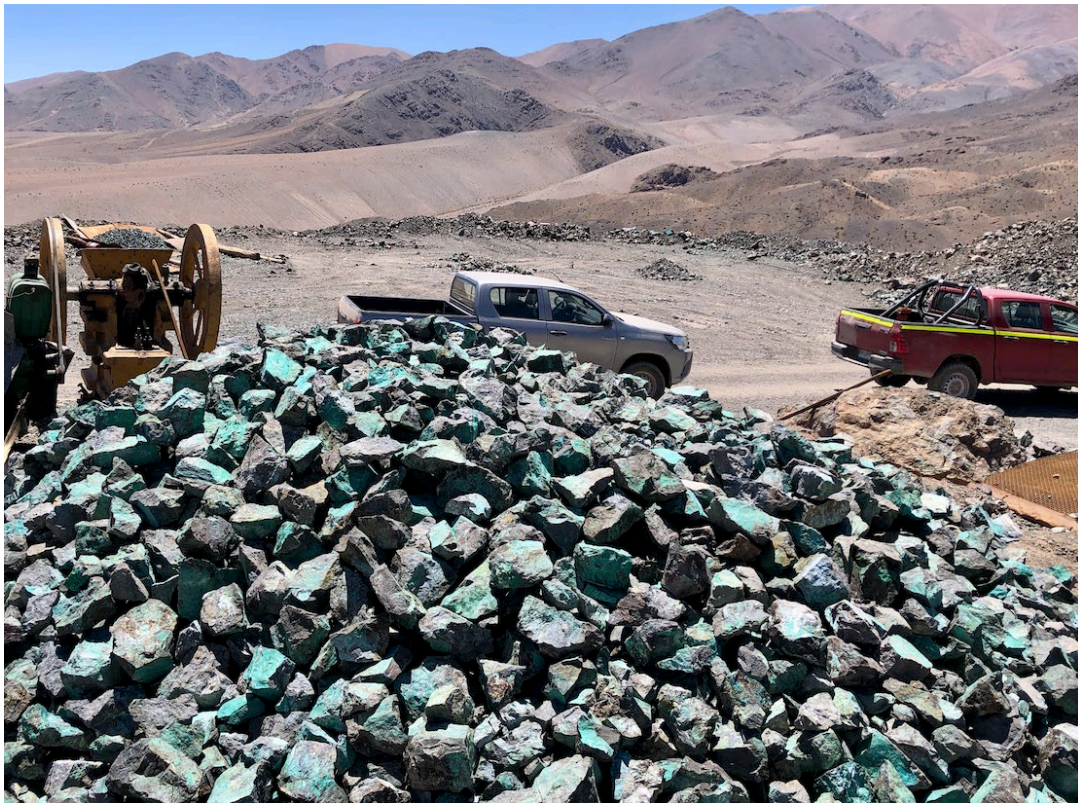
Figure 3: Excavations made by artisanal miners near MODD004 showing the presence of copper oxide mineralisation (green staining)
