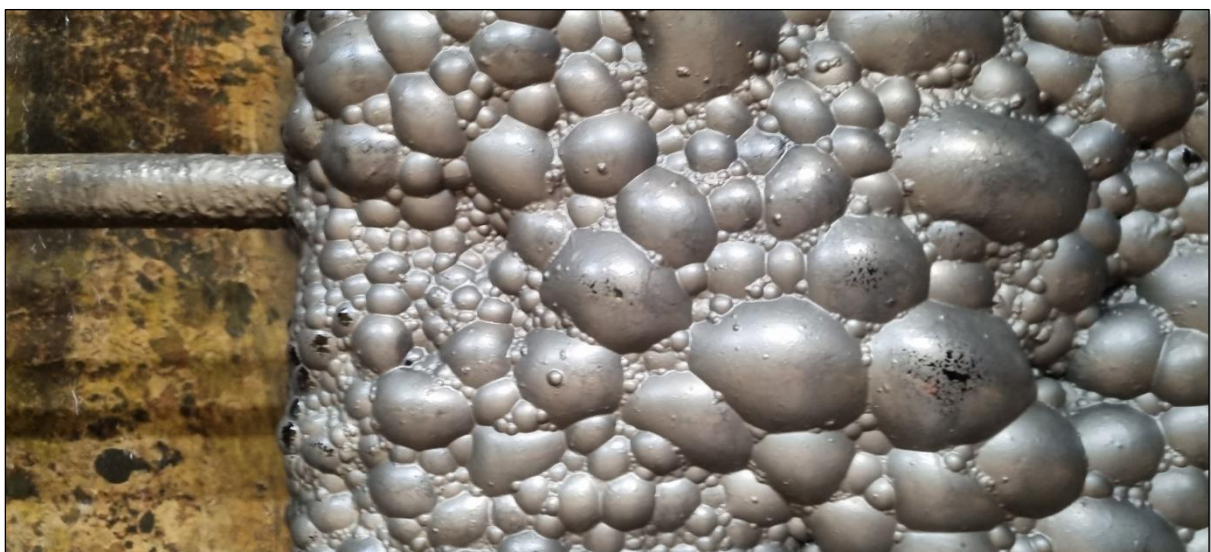
Figure 1 - Nickel Sulfide Flotation, operating at Ban Phuc
