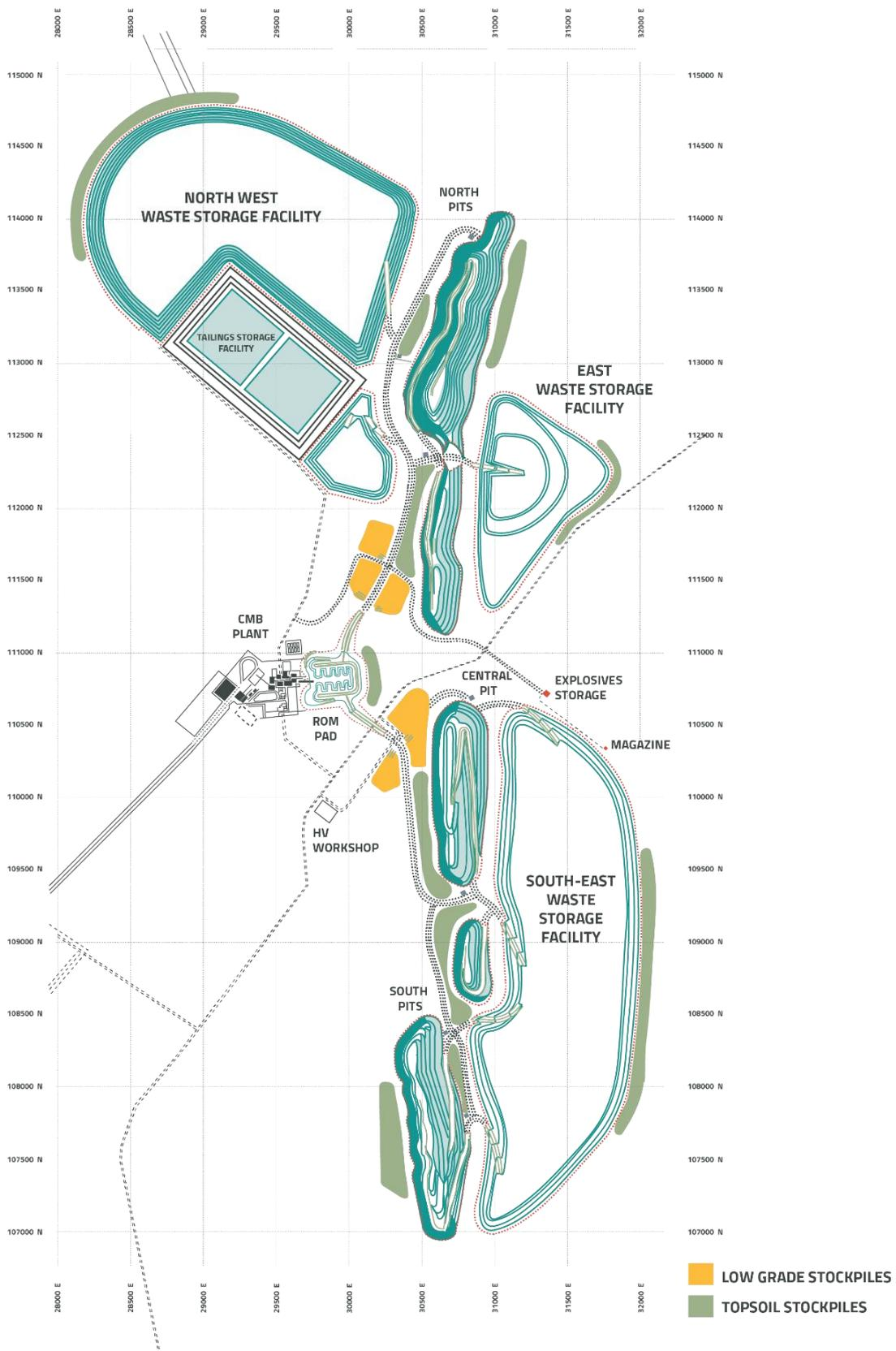
**Figure 11 Site General Arrangement – Plan view including ultimate pits, Waste Storage Facilities, haul roads, ROM pad, long term stockpiles, CMB plant, Tailings Storage Facility, topsoil stockpile locations and public road with proposed diversion**
