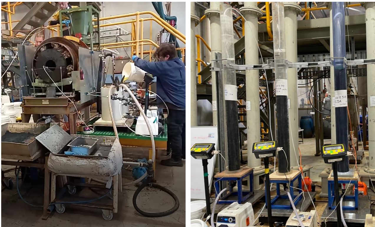
Figure 14 Hydrometallurgy pilot testwork and column wash set-up
