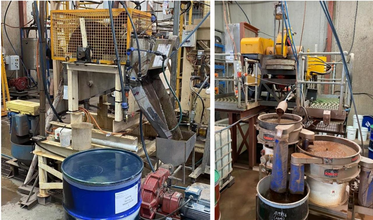
Figure 12 MIMS unit (left) and WHIMS unit (right)
