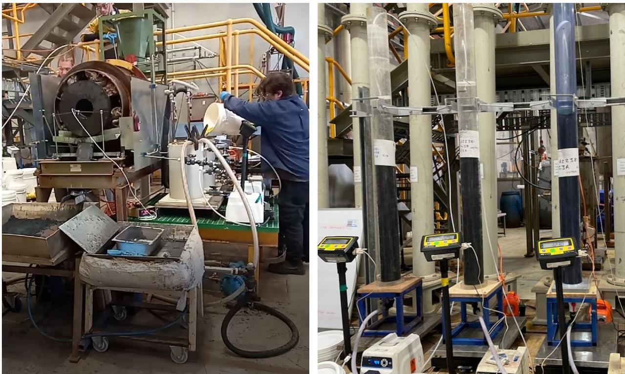
**Figure 14 Hydrometallurgy pilot testwork and column wash set-up**
