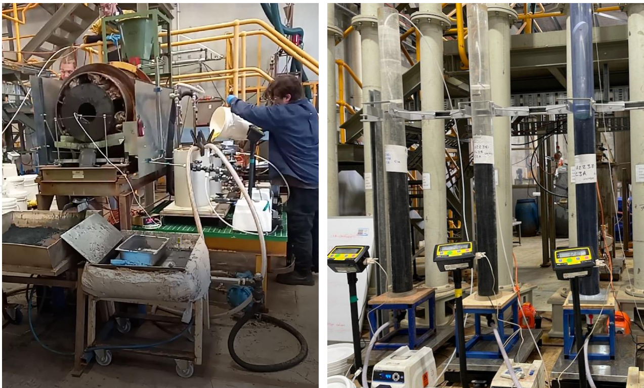
Figure 14 Hydrometallurgy pilot testwork and column wash set-up
