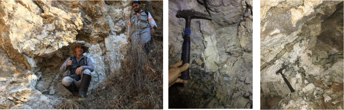
Figure 2: Monte Alto area - Latin Resources geologists mapping outcropping zones with good exposure of large spodumene crystals, kaolinised by surface weathering; and large spodumene identified inside shallow historic galleries/ excavations
