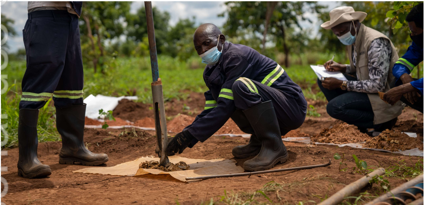
Figure 12: Hand-auger drill sampling and geological logging at Kasiya.
