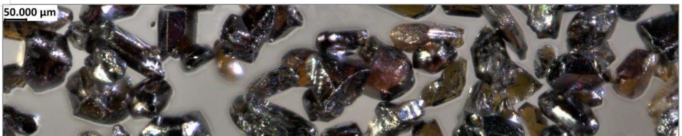
Figure 6: Photomicrograph of high purity rutile product 97.2% TiO 2
