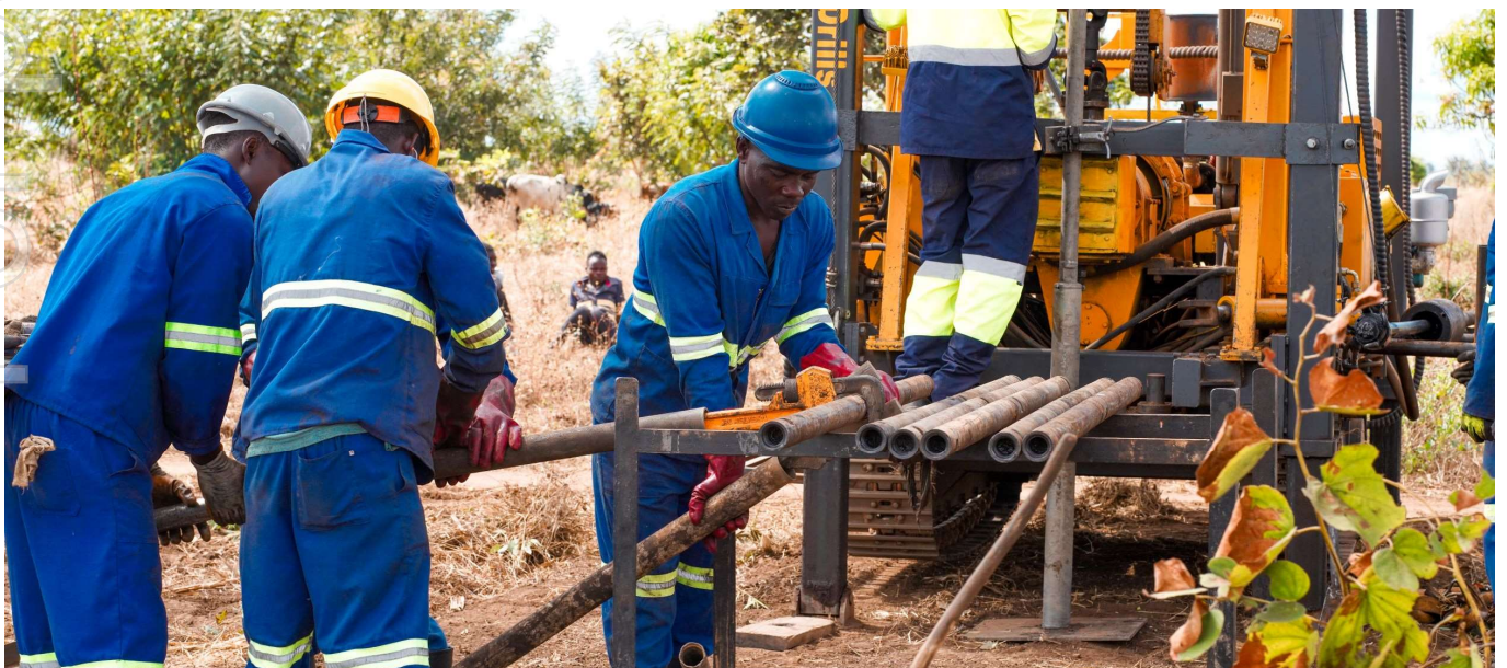
Figure 5: Core drilling at Kasiya
