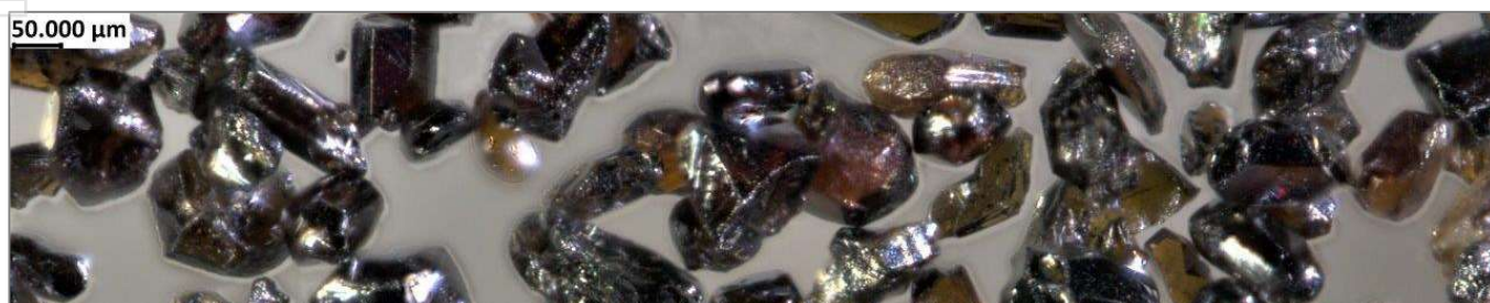
Figure 6: Photomicrograph of high purity rutile product 97.2% TiO 2
