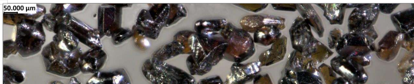
Figure 6: Photomicrograph of high purity rutile product 97.2% TiO 2
