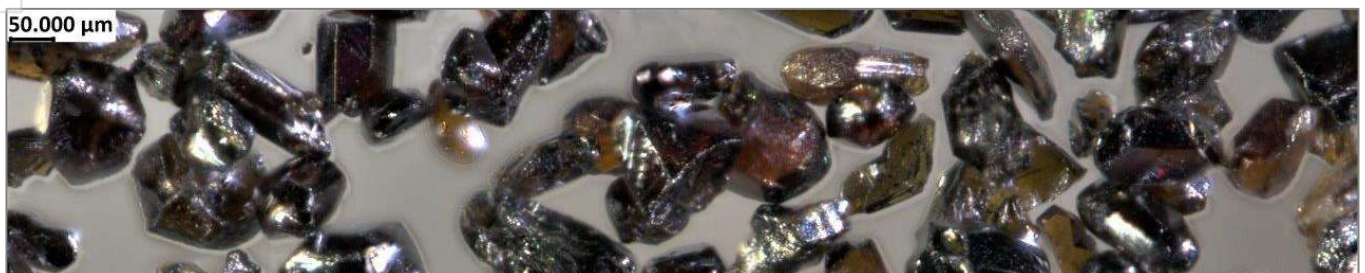
Figure 6: Photomicrograph of high purity rutile product 97.2% TiO 2
