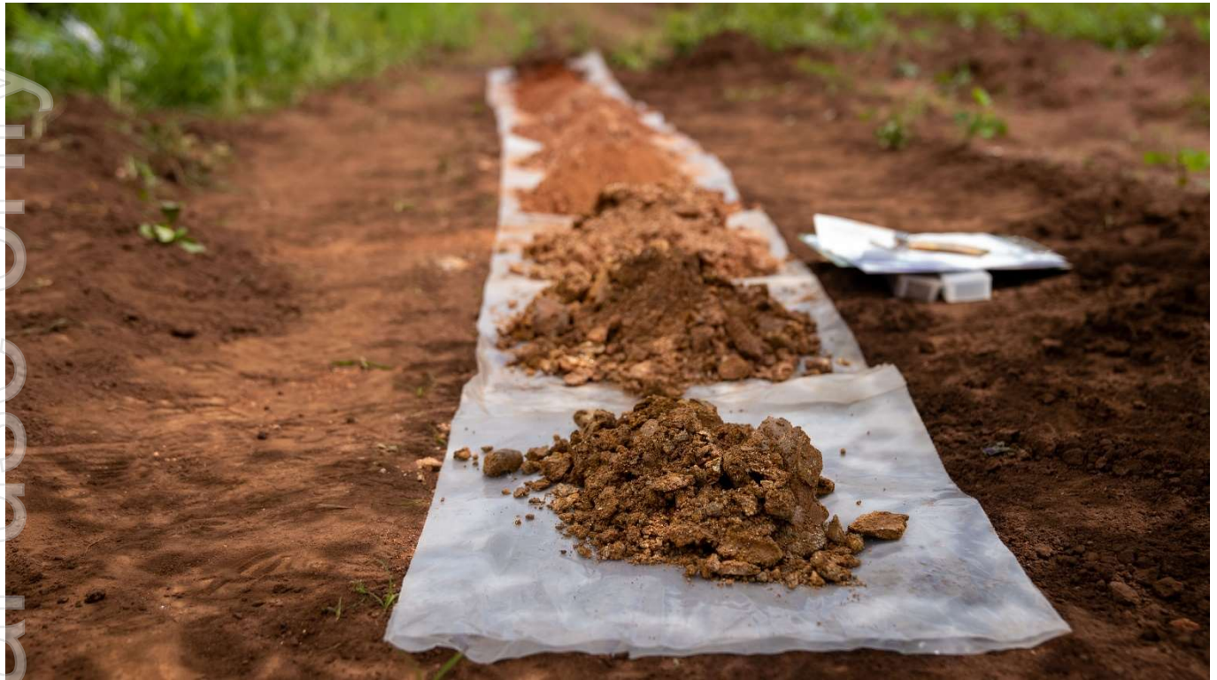
Figure 14: Drill samples prepared for logging
