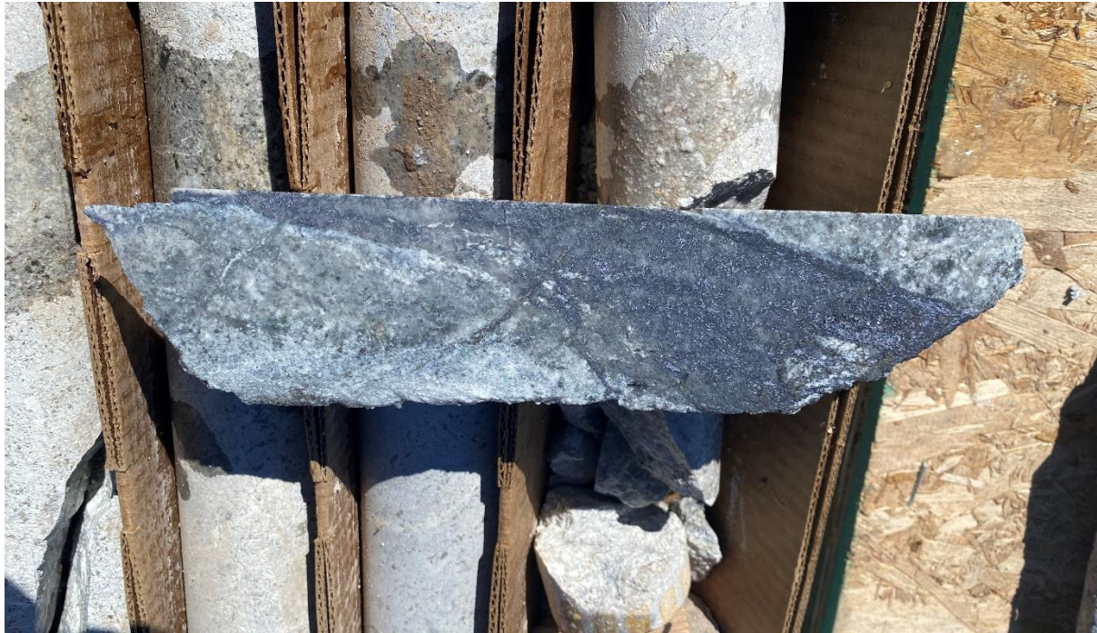
Figure 10: Strong molybdenite, pyrite and quartz veins from WD22-01C at 750m (2460ft).
