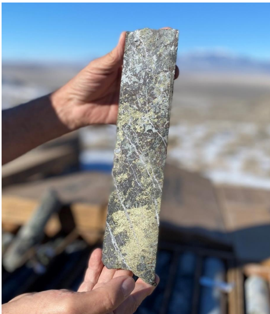
Figure 8: Chalcopyrite rich magnetite skarn in drill core from WD22-01C. The interval is located within the Main Zone of the deposit and from 418m (1,371ft) downhole.
