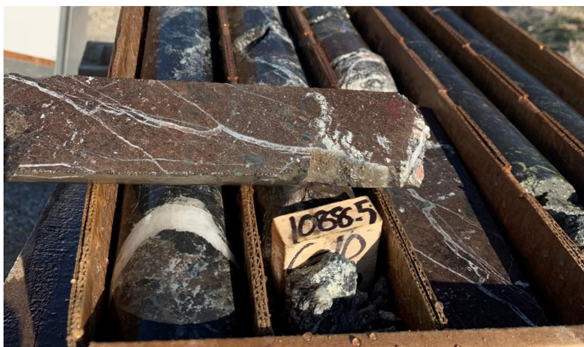
Figure 12: Photo of massive zinc sulphide comprising red-brown sphalerite at approximately 332.8m (1092ft) down hole in drill hole WD22-03. Calcite (calcium carbonate) can be seen as white veins.
