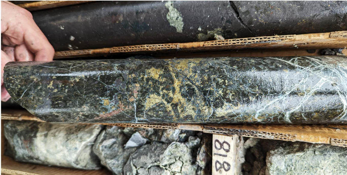
Figure 6: Chalcopyrite and molybdenite rich magnetite skarn in drill core from WD22-01. The interval is located within the Main Zone of the deposit and from 249m (817ft) downhole.
