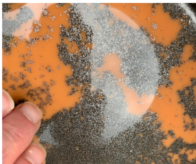
Figures 4 & 5: Very coarse-flake graphite in +600\mu\text{m} sample fraction (L), graphite floating on soaking drill sample (R)
