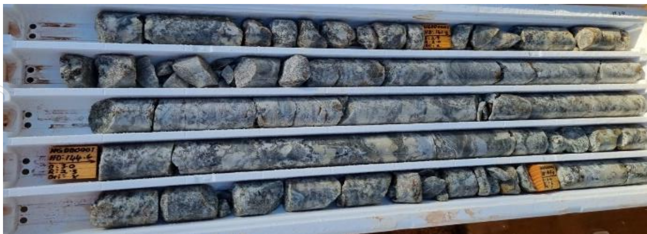
Figure 5 - Intersected pegmatites (86.1 – 94.4m & 131.8 – 146.2m) at the Hilditch Gold Prospect being sampled separately for lithium suite elements (NQ drill hole HGDD001).
