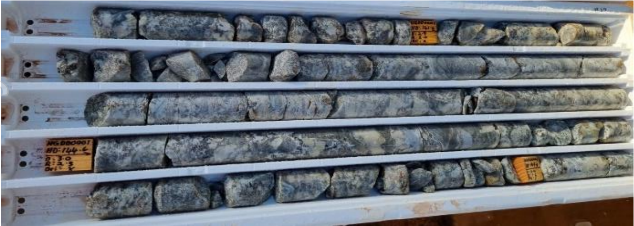
Figure 5 - Intersected pegmatites (86.1 – 94.4m & 131.8 – 146.2m) at the Hilditch Gold Prospect being sampled separately for lithium suite elements (NQ drill hole HGDD001).
