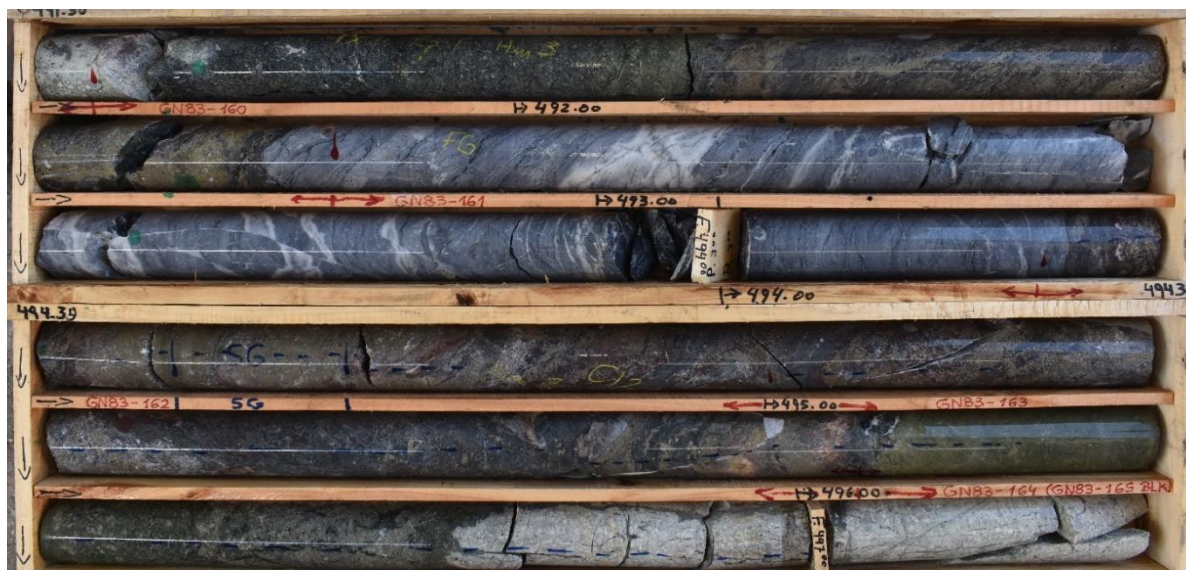
Photo 2 - GNDD-527 : Massive sulphides and skarn alteration logged (491.6-496.8m) showing
