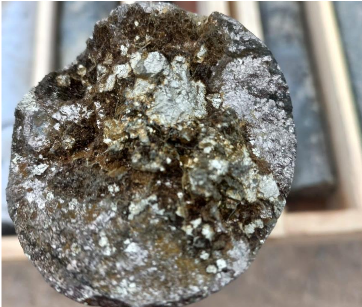
Photo 4 - GNDD-555 : Massive sulphides end of core 496.4 metres downhole
