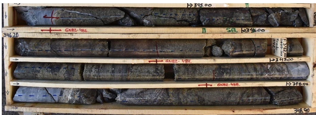
Photo 5 - GNDD-515 : Massive sulphides and skarn alteration logged 345.4-349.1m
