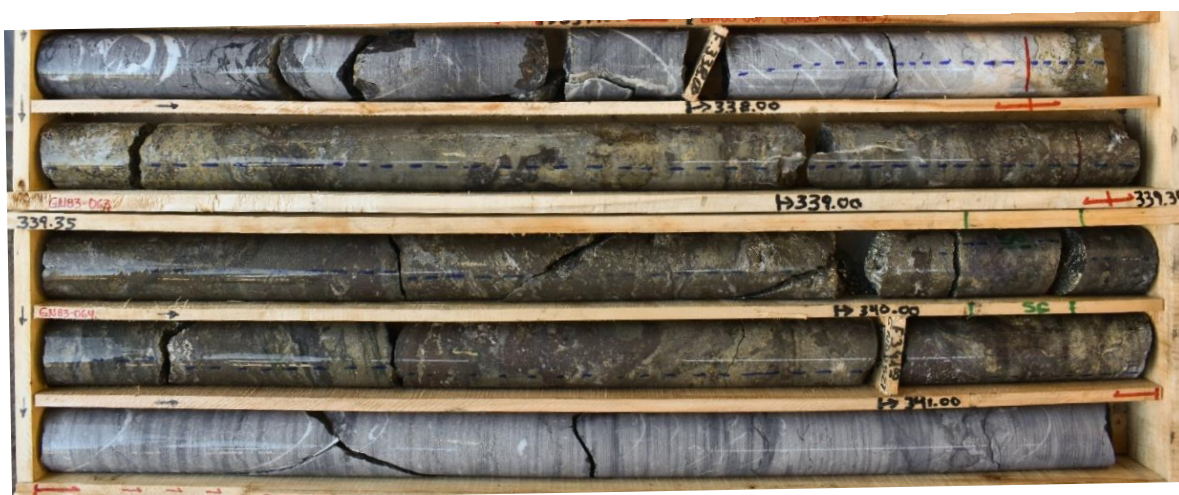
Photo 1 - GNDD-527 : Massive sulphides and skarn alteration logged (338.3-341.3m)
