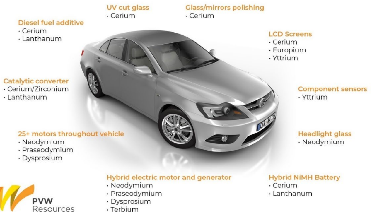
Figure 6: Rare earth elements used in electric vehicles
