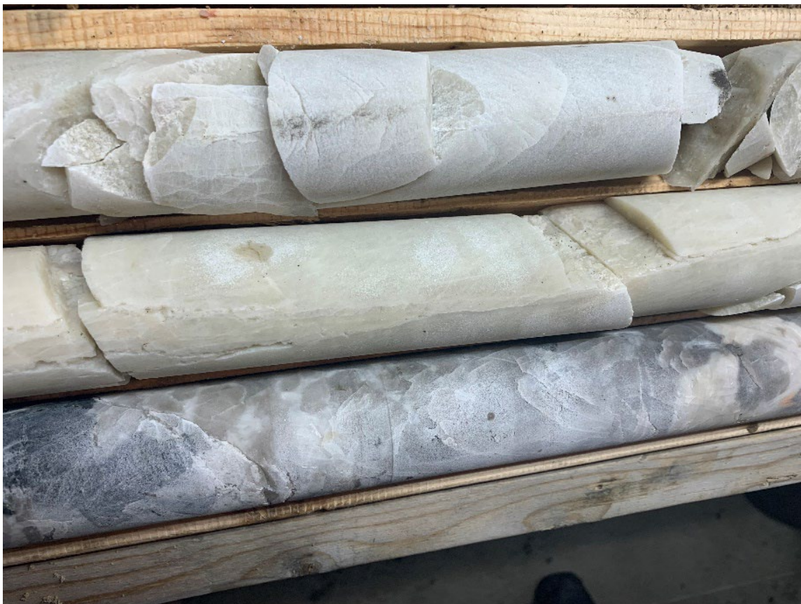
Picture 1 - Visible spodumene crystals have been detected in the initial drill core
