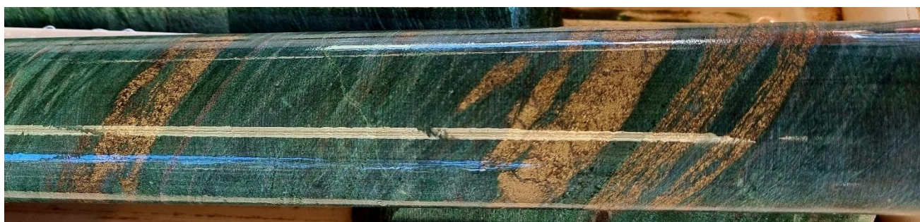
Figure 3. Intense Fuchsite alteration with pyrite in HWDD002 at 179.7m
