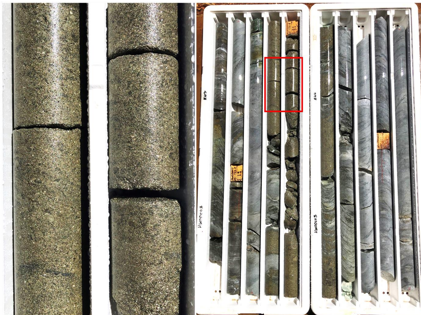
Figure 4. Massive pyrite in HWDD003, between 154.2 and 156.6m. Wall rocks are intensely silicified metasediments. Red box indicates area enlarged on the left-hand side.
