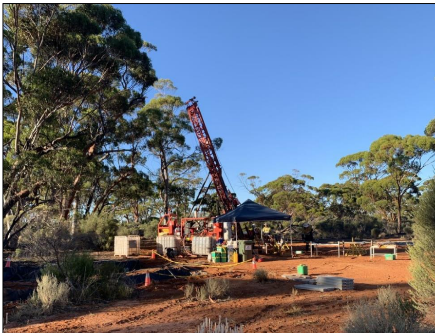
Figure 3 - Diamond Drill Rig at the Godley Target - NRDD0001
