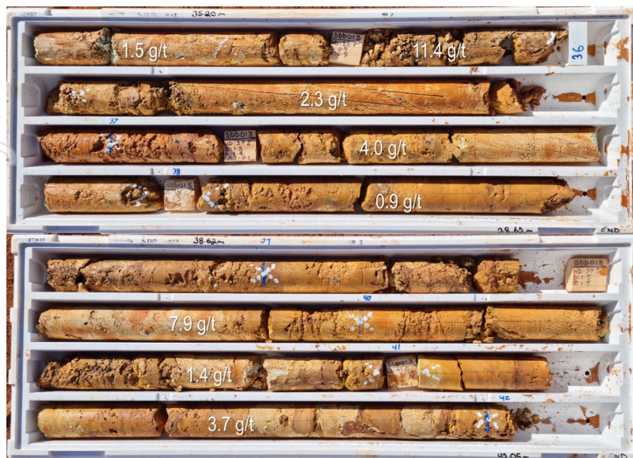
Figure 10. Diamond core from SDD013 from 35.20m to 42.05m HQ (63mm diameter). (Table above) Summary assay table for SDD013 from 29.4m to 49m
