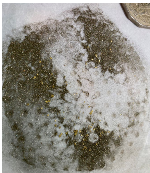
Plate 2 – Gravity gold concentrate obtained from a 5kg – 15g/t Au transitional basalt sample rod milled to P80 passing 75 micron then gravity concentrated – via Knelson centrifugal concentrator (phase 1) and the Mozley Table (phase 2); large nuggety gold grains visible in concentrate. Larger grains flattened due to rod milling process.
