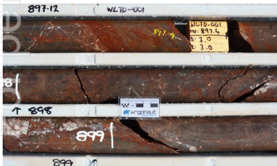
Photo 2. WLTD002, 770.5m to 772.7m, Murdie project: IOCG-style hematite alteration and brecciation.
