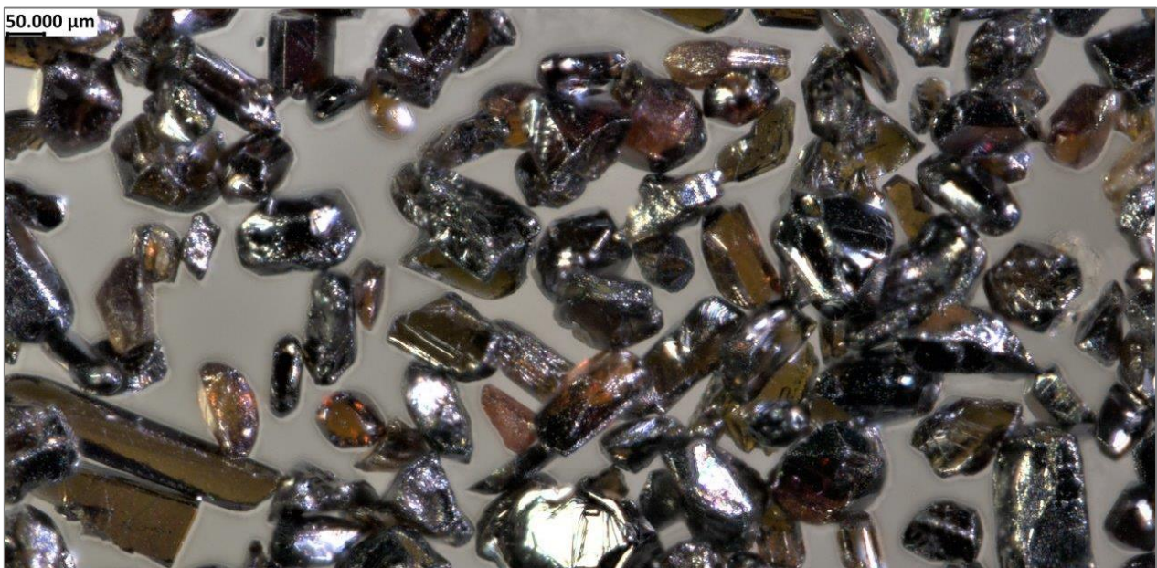
Figure 9: Photomicrograph of high purity rutile product 97.2% TiO 2 .
