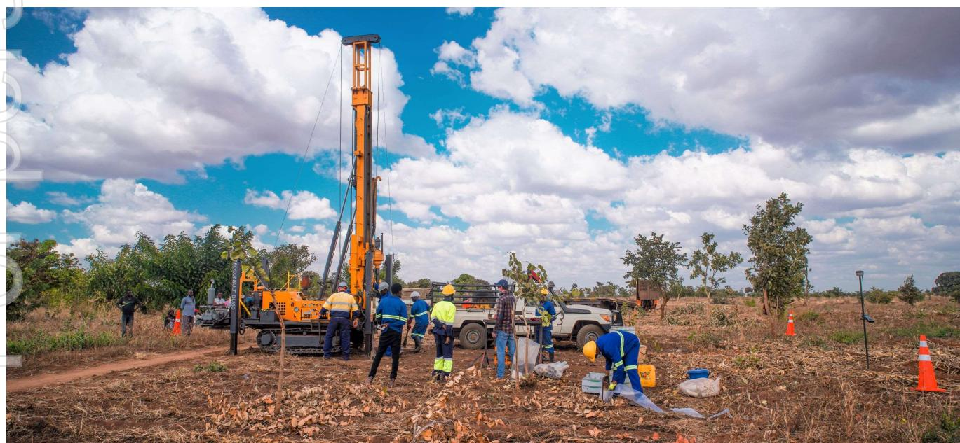
Figure 2: DL650 push-tube core drilling rig in operation at Kasiya-Nsaru
