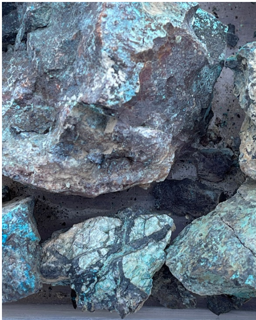
Figure 3. Sample NSM-21-032: 16.8% Cu and 8.48g/t Au (772413E, 3781087N)
