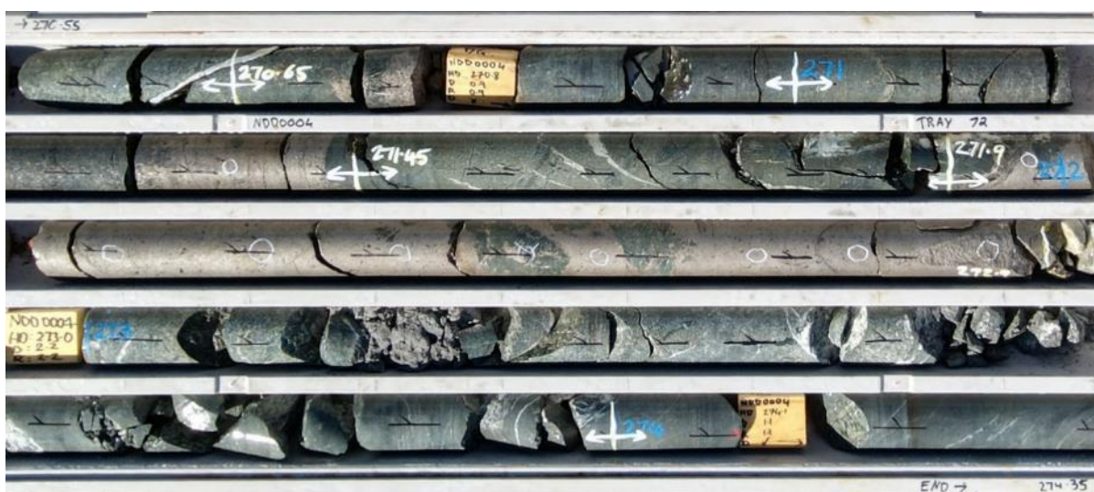
Figure 8. Massive sulphide intersected by NDD0004, which returned an average grade of 1.35% Ni.
