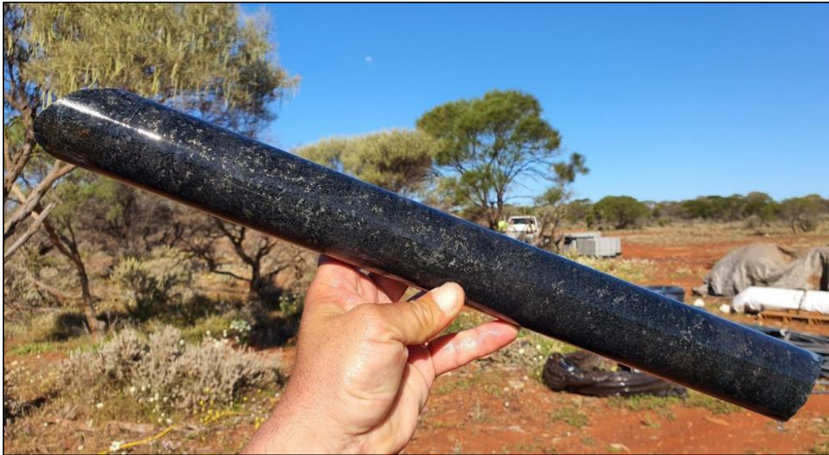
Figure 3. Cumulate-textured high-MgO ultramafic with disseminated and blebby magmatic sulphides from 89m in NDD0008.
