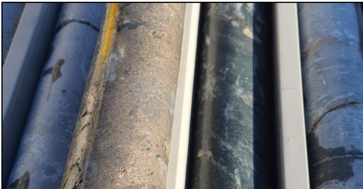
Figure 9. Semi massive and disseminated sulphide intersected by NDD0010 around 140m downhole. The hole size is NQ2.
