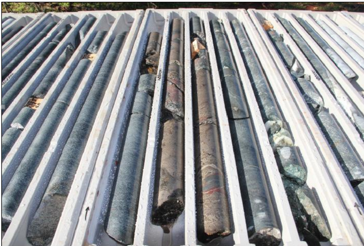
Figure 2. Photograph showing massive and semi-massive sulphides intersected by NDD0001 from approximately 212.7m. pXRF readings were used to confirm the presence of nickel, copper, and cobalt.
