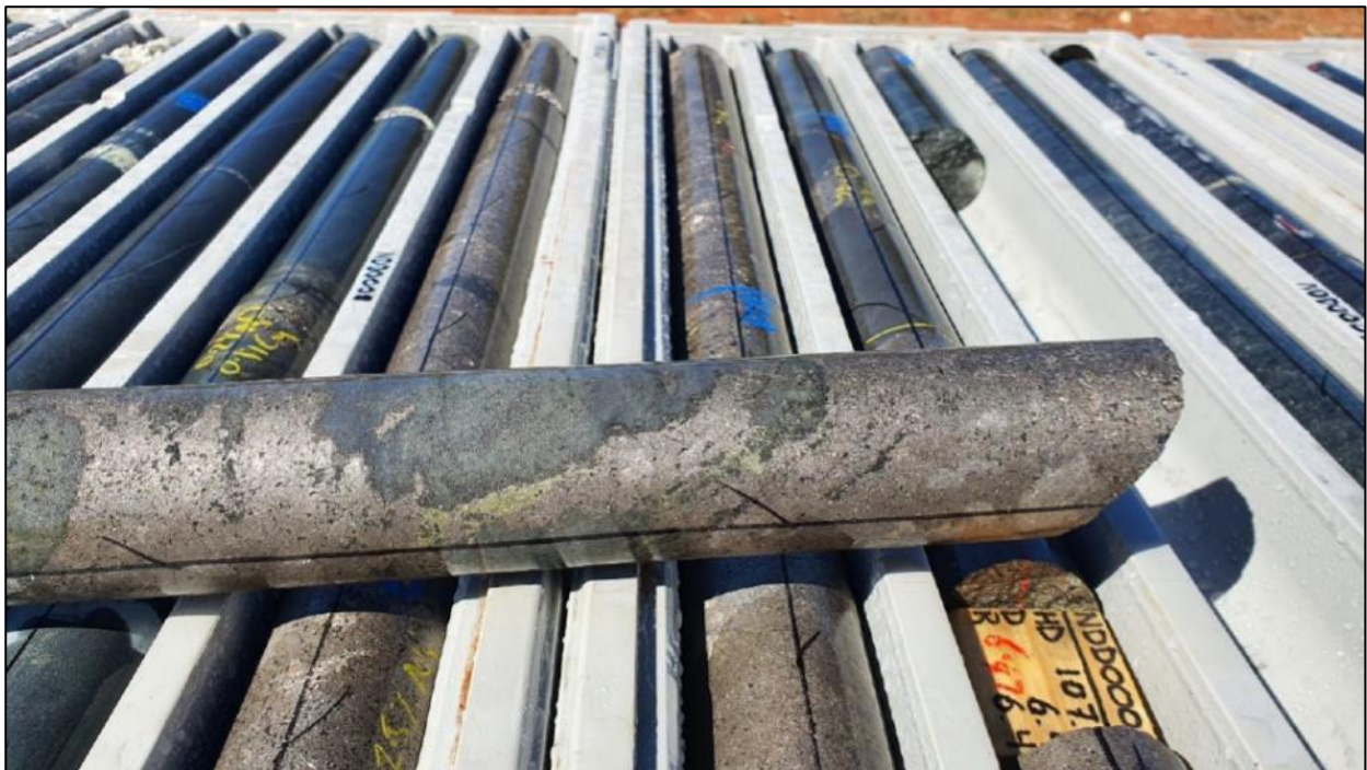
Figure 4. Semi-massive sulphide from approximately 106m downhole in NDD0008, showing the interaction of the sulphides with country-rock xenoliths and clots of remobilised chalcopyrite.
