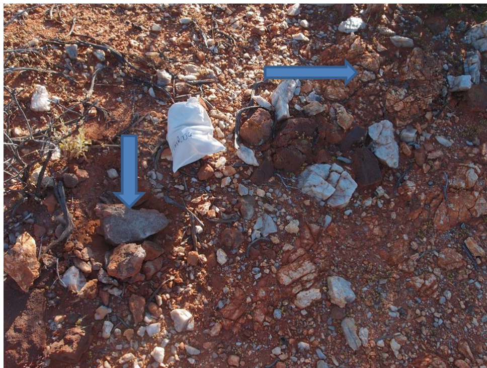
Figure 18. Rock sample NR0004, grisen-like morphology consisting of micaceous laths and microcline. Laboratory analysis reported 9,307ppm Rb and 0.32%Li and 1,934ppm Cs. Arrows indicate the sample outcrop and rock texture on a fresh face.
