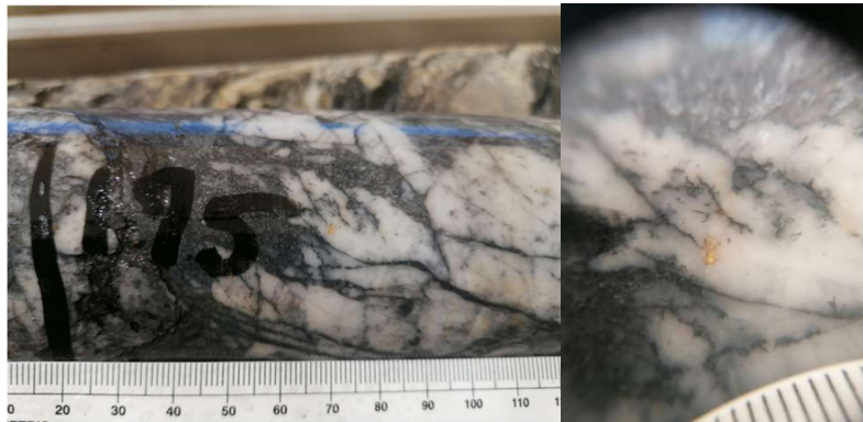
Figure 9: Visible Gold intersected in ore zone
