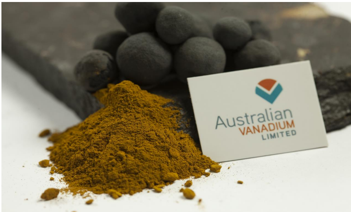
Figure 3 - Sample of V 2 O 5 precipitate generated from pilot program alongside roasted pellets and a vanadium ore sample
