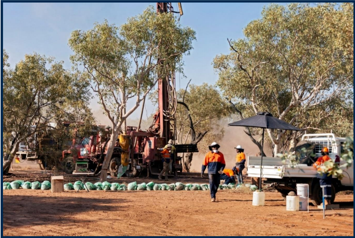
Photo 1: Reverse circulation drill hole (HERC003) in progress at Hermitage. Note sand cover and lack of surface expression of the ironstone which hosts the mineralisation some 75m below the surface.
