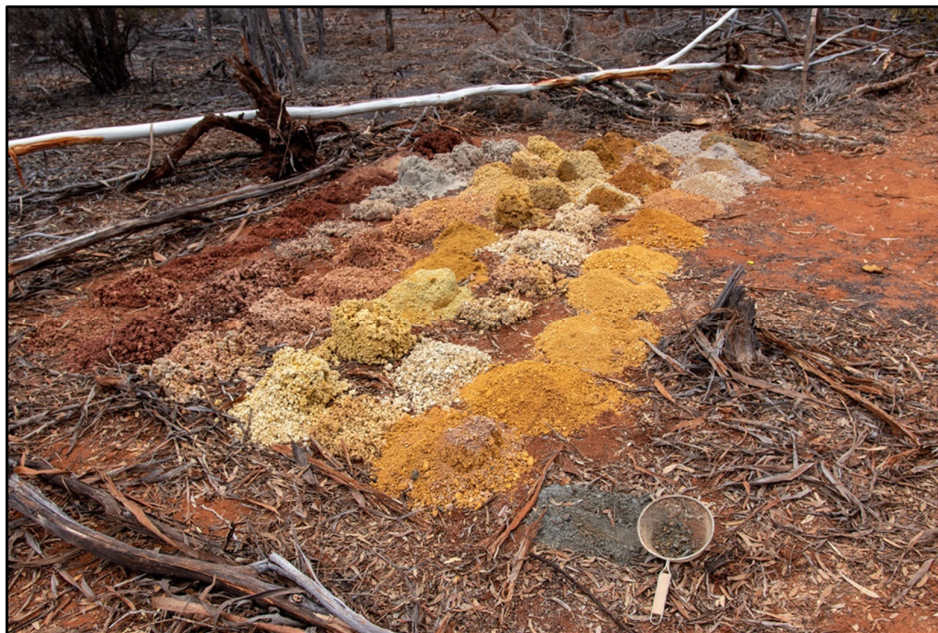
Figure 10 —Aircore Drill Samples with 1 Metre of Sulphide at End of Hole (right foreground with sieve)
