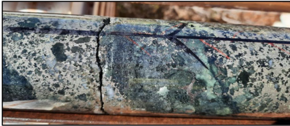
Figure 5 - Matrix sulphide mineralisation at 399m downhole in DBDD001 (field of view approximately 20cm across)
