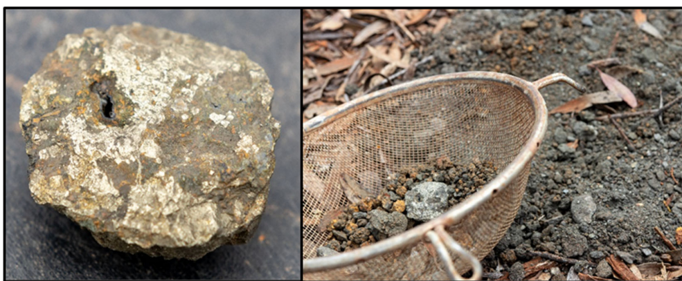
Figure 9 – Massive Sulphide Chip (25mm across) from 60m in NAC105. Bottom of Hole Sample Pile on Right. Drillhole was Unable to Breakthrough Sulphide
