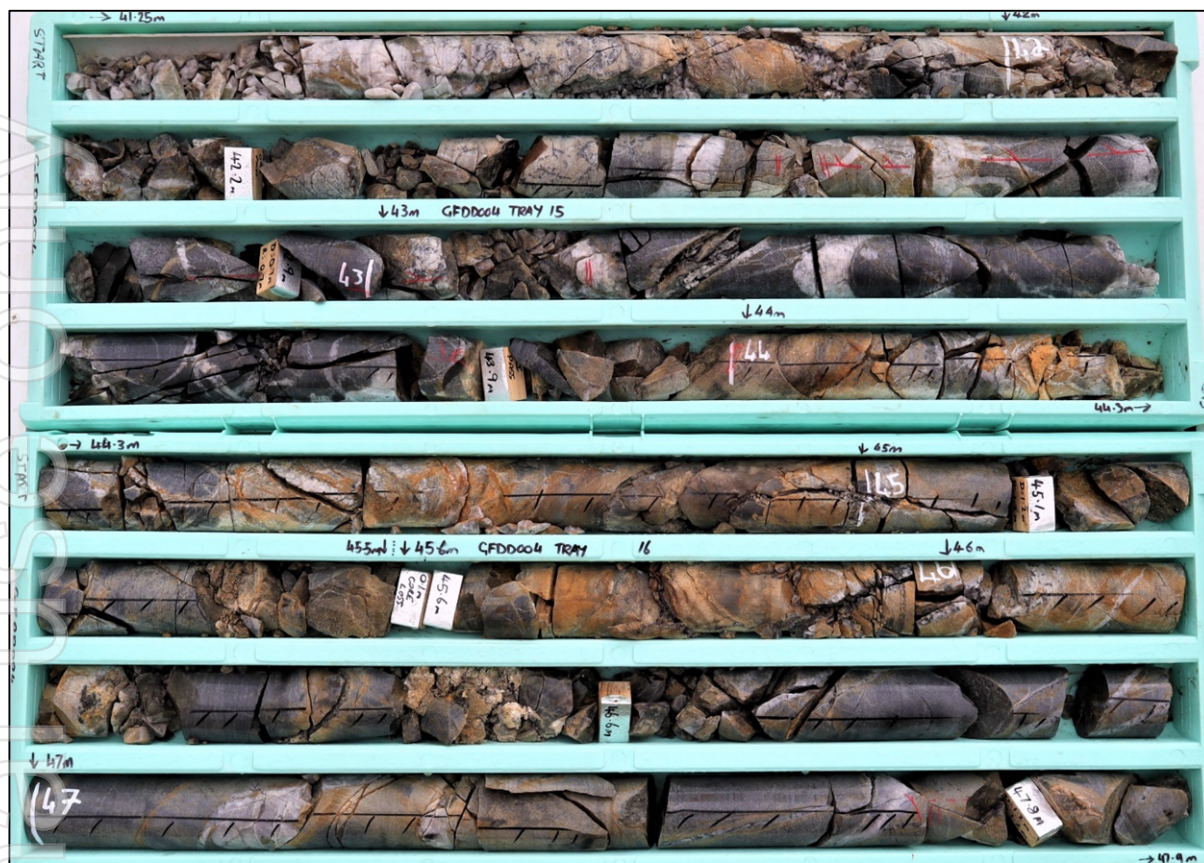
Figure 11: Photograph of drill core from GFDD004, Grand Flaneur prospect, showing quartz-sulphide veining in strongly ferrous carbonate altered silicified channel sand host unit. Interval shown includes 1.4m @ 9.66 g/t Au from 45.6m .
