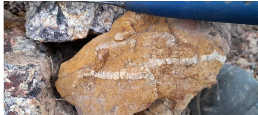
Remnant porphyry A-veins overprinted by phyllic alteration
