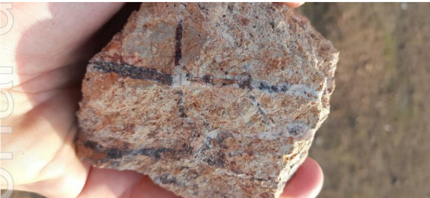
Remnant porphyry B-veins in diorite overprinted by phyllic alteration
