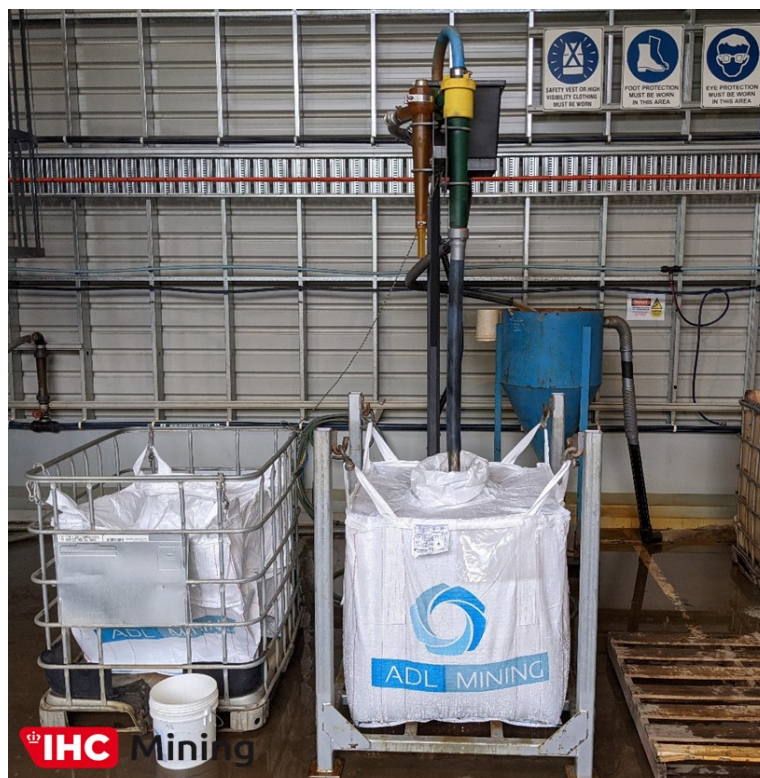
Plate 4 – Slimes removal (material <45\mu\text{m} )
