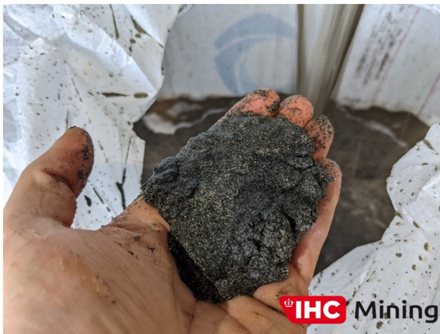
Plate 5 – Washed sand ready for industrial sand and magnetite-heavy mineral recovery (+2mm -45µm)
