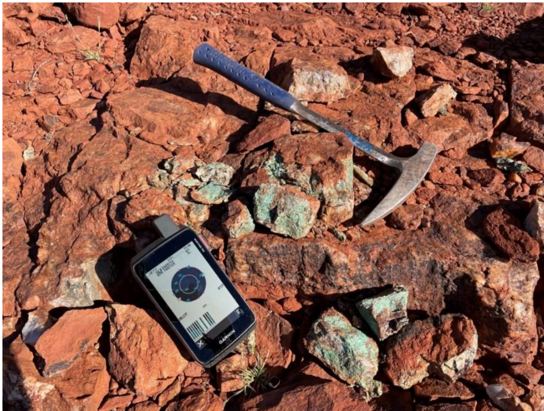
Figure 16: Malachite-rich sample BLGS0217 (5.73% Cu and 5.74 g/t Au) from infill sampling at Eagles Rest.
