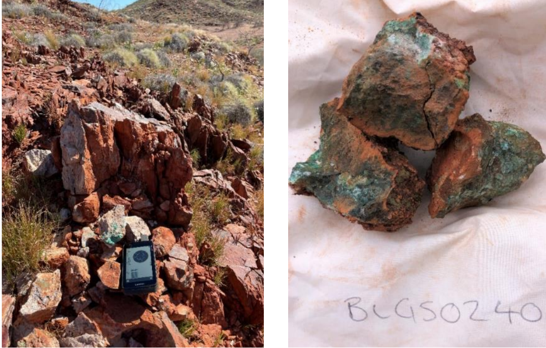
Figure 12: Outcropping mineralisation at the newly discovered Green Hills Prospect and rock chip sample BLGS0240 which returned results of 24.30% Cu and 0.59 g/t Au.
