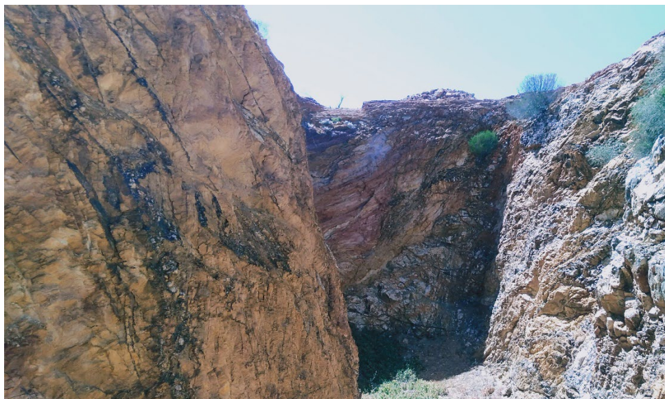
Figure 4 – Linger and Die Well Pit - looking east – note quartz veining in main face and south dipping veins in northern wall
