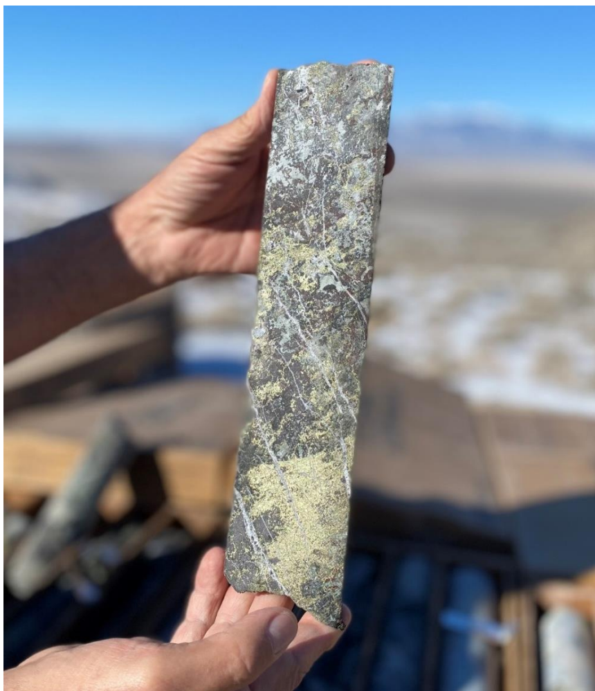
Figure 1: Chalcopyrite rich magnetite skarn in drill core from WD22-01C. The interval is located within the Main Zone of the deposit and from 418m (1,371ft) downhole.
