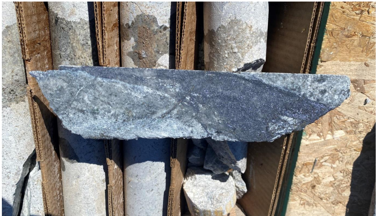
Figure 4: Strong molybdenite, pyrite and quartz veins from WD22-01C at 750m (2460ft).
