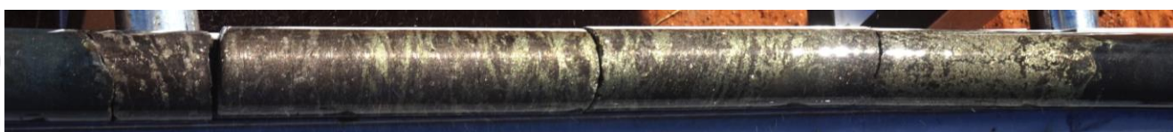
Figure 2. High grade massive sulphide from PSD02. The sulphide has a conductance in excess of 5,000 siemens and similar to that modelled for the new conductor.
