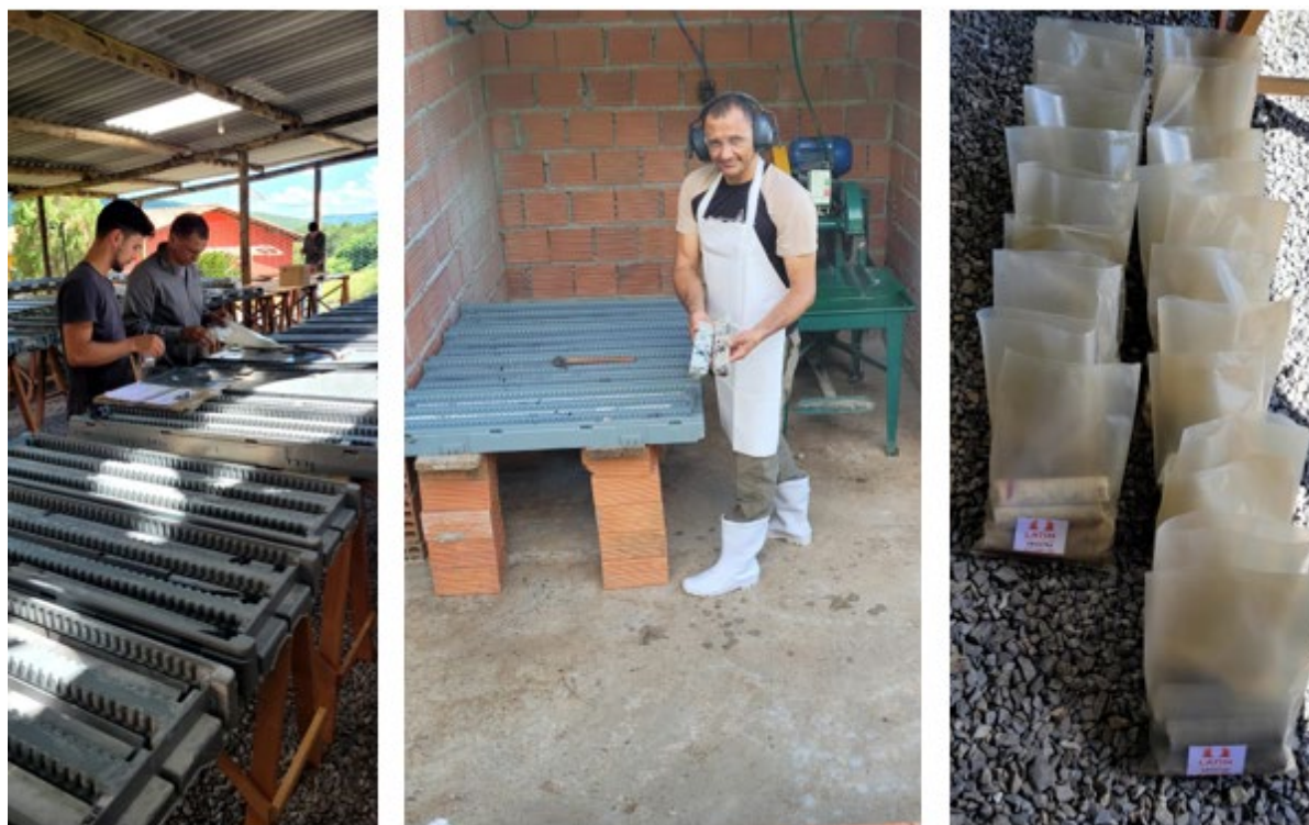
Figure 6: Drill logging, core cutting and sampling on site at the Salinas Lithium Project, Brazil
