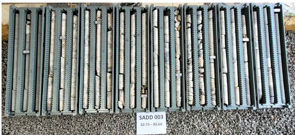
Figure 1: SADD003 – spodumene bearing pegmatite 65.6-81.77m, (16.17m true thickness) intersected in diamond drilling approximately 180m along strike to the south of previously reported intersections 1
