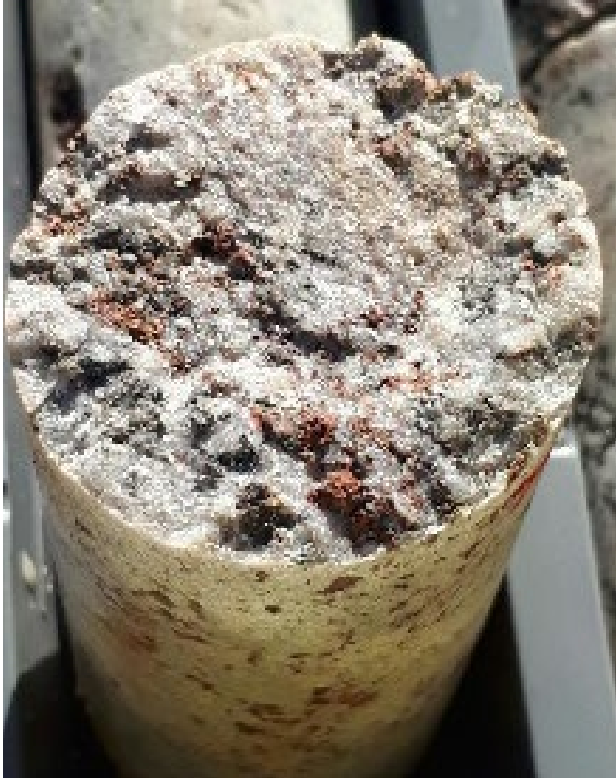
Figure 4 Figure 4: Brick red coloured coarse grained disseminated REE minerals at 748m depth-ankerite carbonatite host rock. The sample is part of a 4m composite from 747m to 751 has assayed 2.44% REO
