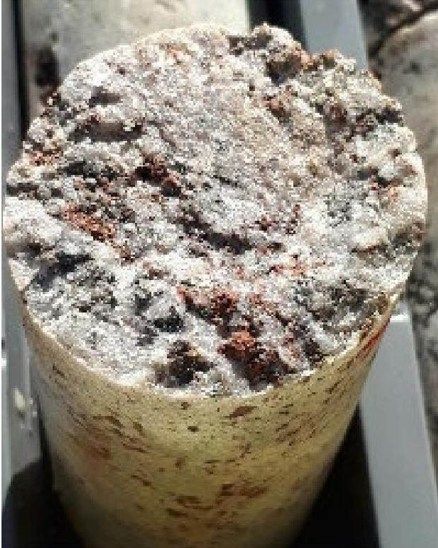
*Figure 4 Figure 4: Brick red coloured coarse grained disseminated REE minerals at 748m depth-ankerite carbonatite host rock. The sample is part of a 4m composite from 747m to 751 has assayed 2.44% REO*
