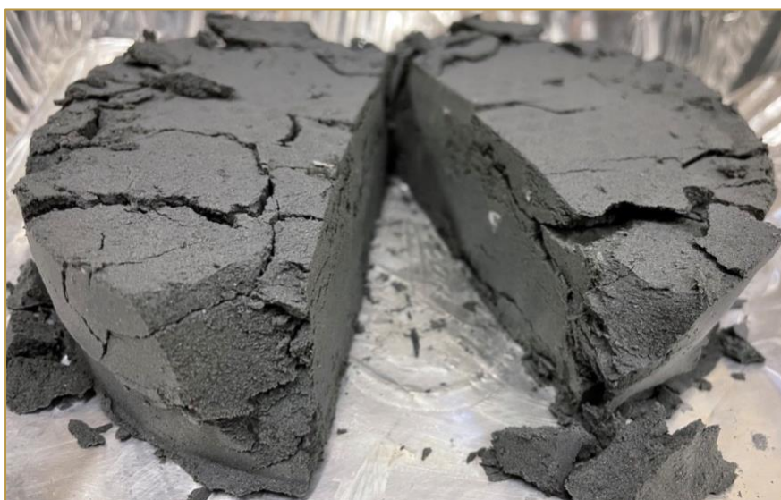
Figure 6-4, Tailings Filter Cake (16.6% moisture, w/w)
