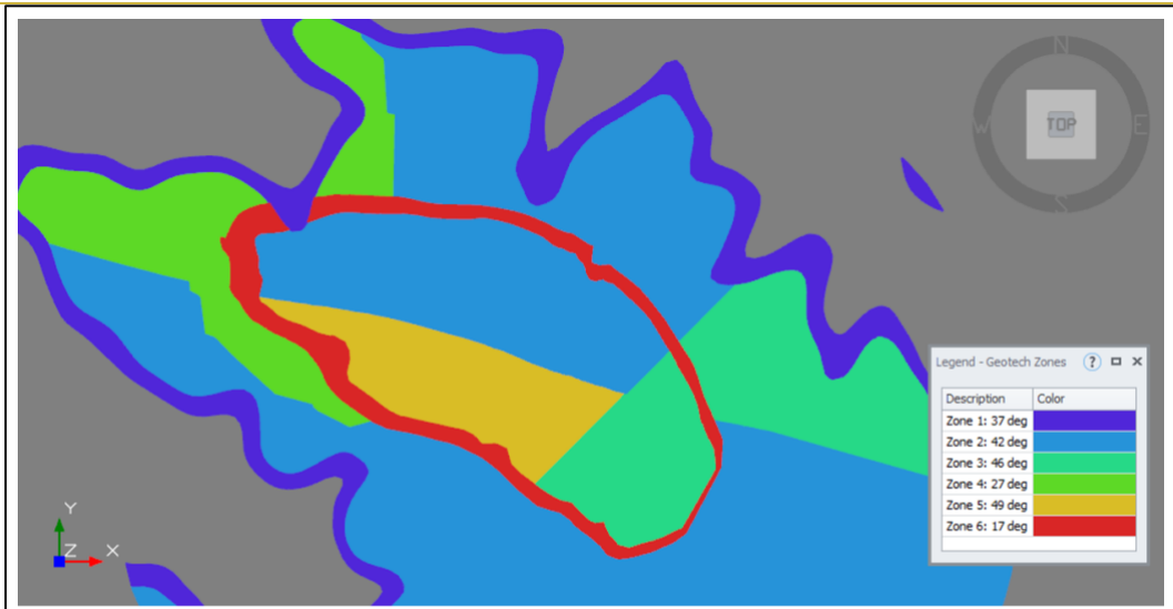
Figure 4-1: Design Pit Slopes by Zone (plan view)
