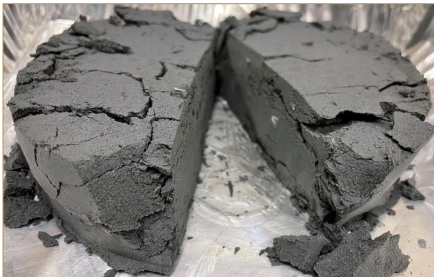
Figure 6-4, Tailings Filter Cake (16.6% moisture, w/w)
