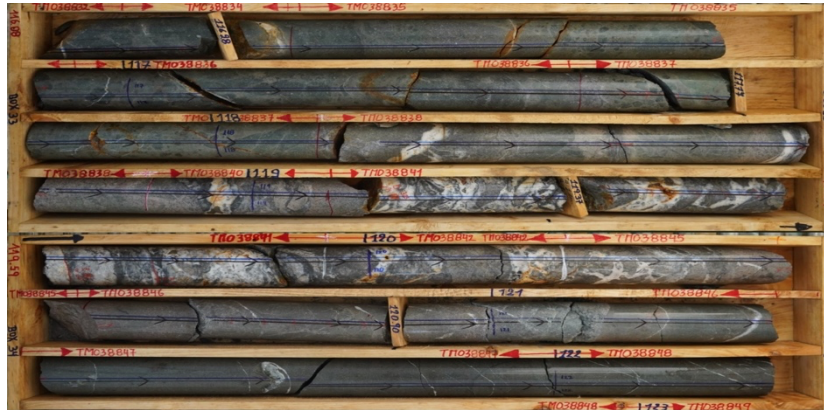
Figure 4: A photograph of mineralised interval in borehole CVD085, averaging 3.08g/t gold over 5.18m from 116.17m. The mineralised interval is centred around a 1.64m quartz-carbonate breccia averaging 5.74g/t gold which is bounded by a phyllic alteration halo.
