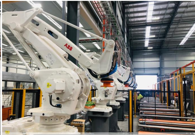
6 robots capable of delivering a pallet of finished goods out of production every 2 minutes
