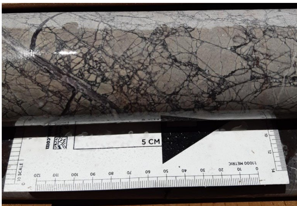
Figure 1: Brecciated fine-grained diorite with chlorite +/- pyrite-chalcopyrite-bornite fracture fill (MODD003: 362m)
