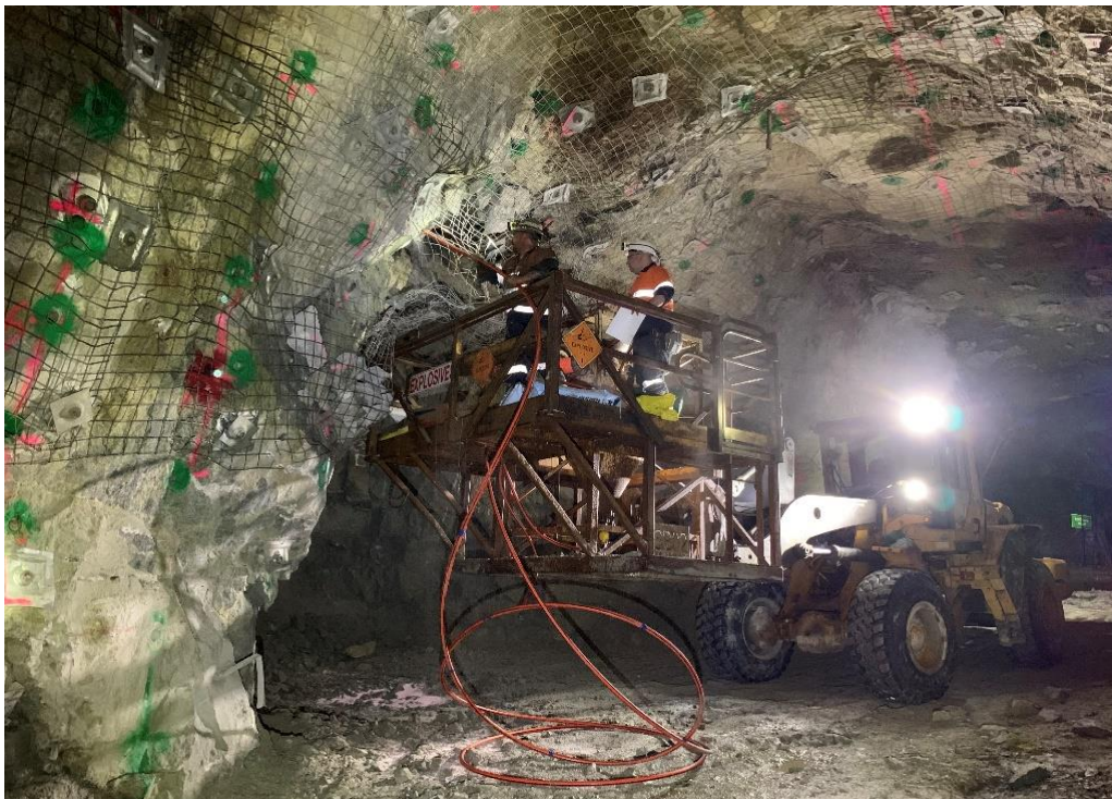
Figure 1: Kaiser employees charging the first production hole of the Queens Lode ore body, with firing recently completed.
