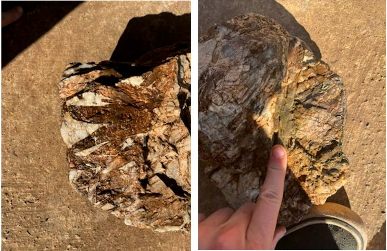
Figure 2: LCT Spodumene lithium mineralisation at Big pegmatite
