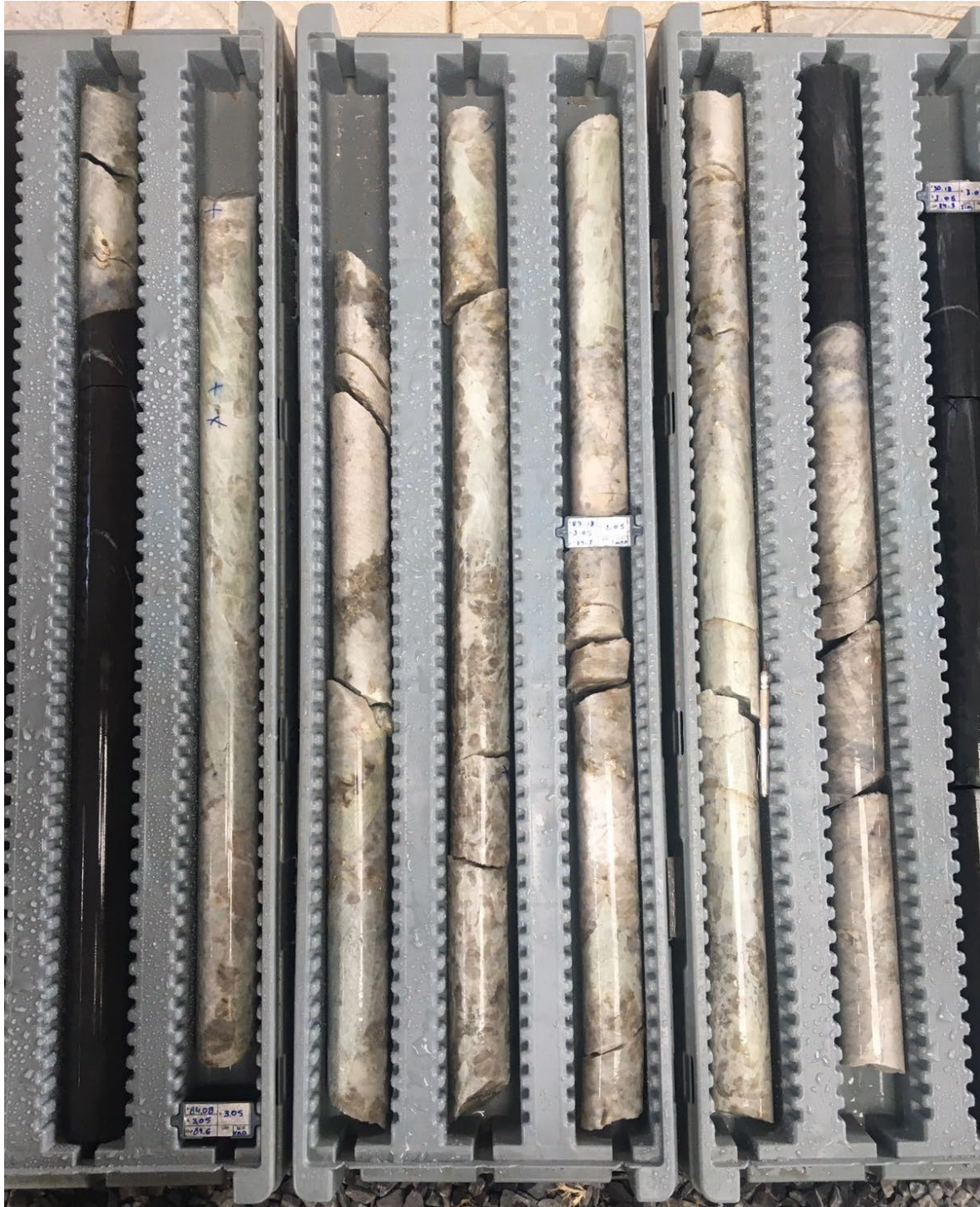
Figure 2: SADD001 - 5.25m thick coarse-grained pegmatite (83.85-89.10m), containing light green spodumene crystals, hosted within a biotite-quartz schist (black rock) (Refer Appendix 1) 2
