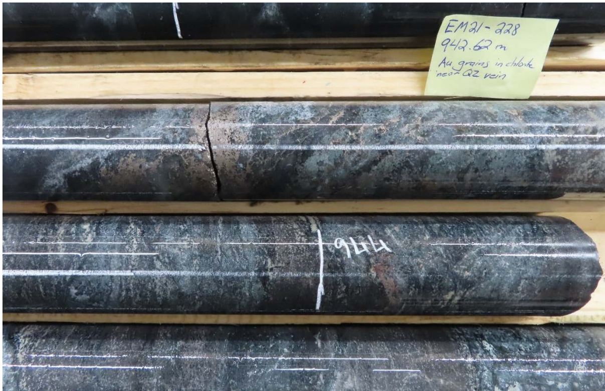
Figure 2: Mineralised interval with alteration, quartz veining and pyrrhotite mineralisation, EM21-228 ~944m. Pyrrhotite is the iron sulphide detected by electromagnetics.
