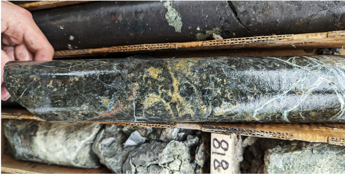
Figure 1: Chalcopyrite and molybdenite rich magnetite skarn in drill core from WD22-01. The interval is located within the Main Zone of the deposit and from 249m (817ft) downhole.
