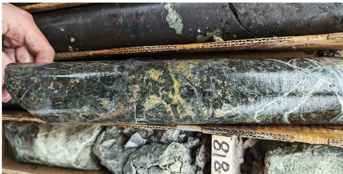
Figure 1: Chalcopyrite and molybdenite rich magnetite skarn in drill core from WD22-01. The interval is located within the Main Zone of the deposit and from 249m (817ft) downhole.
