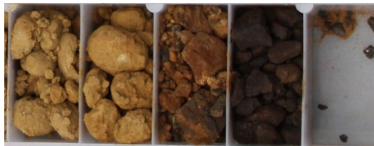
Image 6 / RC drill chips: 21MDRC017 34-39m (5m @ 1.68% Cu & 678ppm Co cuprite mineralisation)
