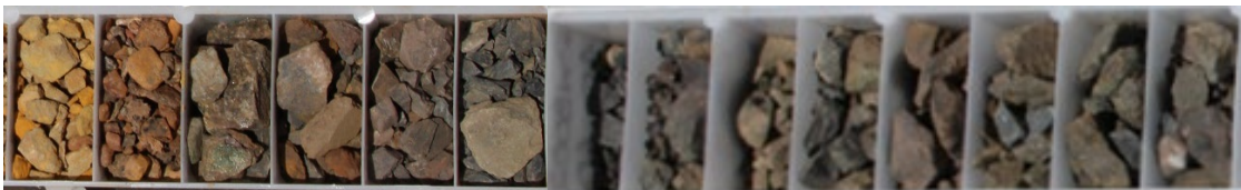
Image 8 / RC drill chips: 21MDWB02 34-48m (14m @ 0.81% Cu & 366ppm Co. malachite & cuprite mineralisation)
