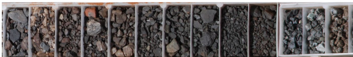
Image 3 / RC drill chips: 21MDRC012, 50-63m (13m @ 0.85% Cu & 429ppm Co, cuprite, chalcocite & covellite mineralisation)
