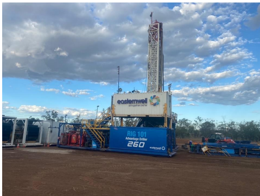
Easternwell Rig #101 being set up at Wellesley-2 drill site
