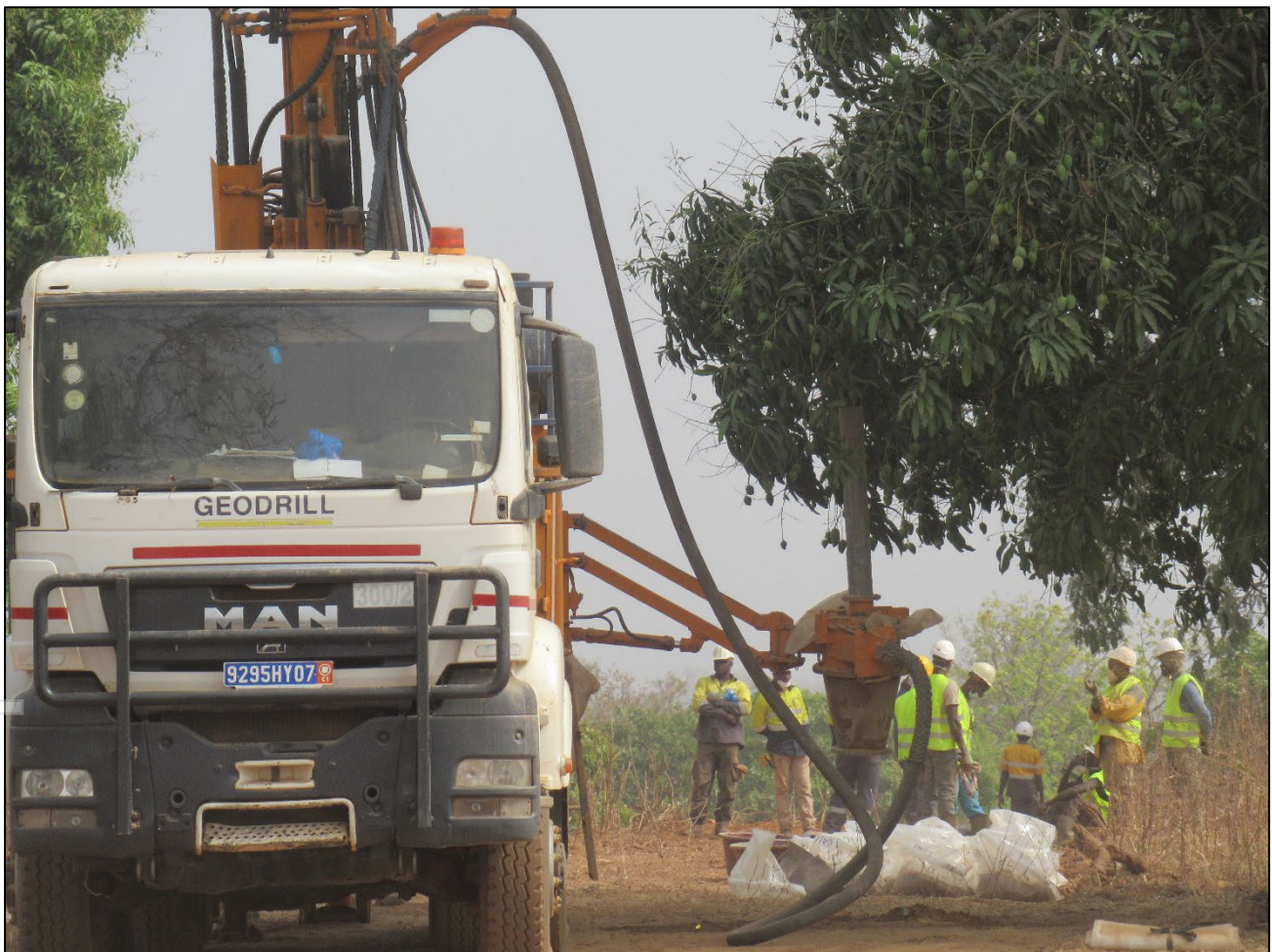
Figure 2: Aircore drilling in progress on the Komboro Prospect (Napié Project)
