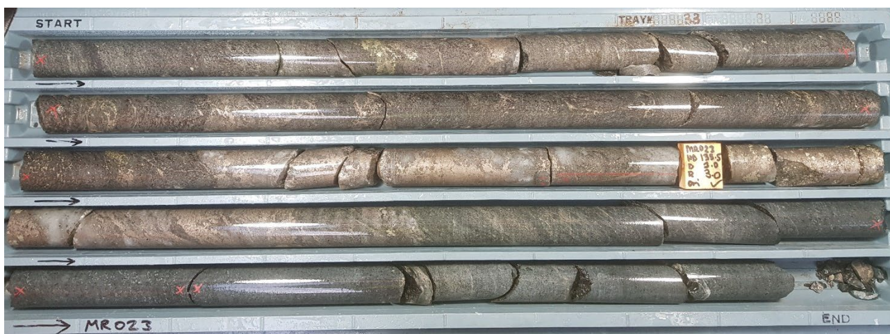
Figure 1: DD22MR023: Pyrite-pyrrhotite-chalcopyrite mineralisation from approximately 131.5m downhole
