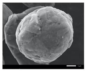
Scanning electron microscopy of high purity alumina doped coated spherical graphite.
