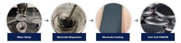
Electrochemical performance of the coated spherical graphite (coated anode) and HPA-doped coated spherical graphite (HPA-doped coated anode) was undertaken in an industry standard coin cell (CR2016) to determine the performance in a lithium-ion cell which are used to power EV's.
