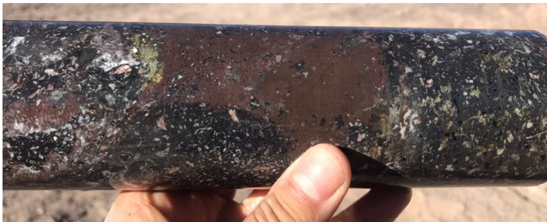
Figure 4: Mostazal Copper Project – diamond drill core from MODD001, showing altered porphyritic andesite host rock with disseminated and clotty sulphide mineralisation, including pyrite and chalcopyrite (copper sulphide)
