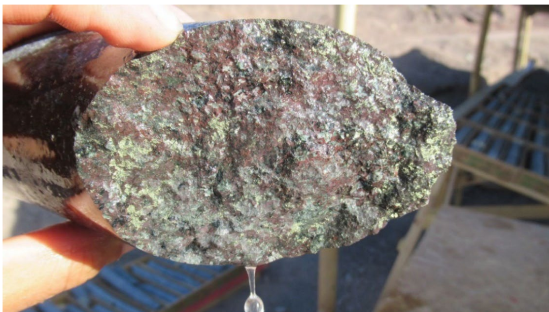
Figure 1: Altered andesitic basalt with fine grained disseminated pyrite and chalcopyrite (copper sulphide) ( MODD002 )
