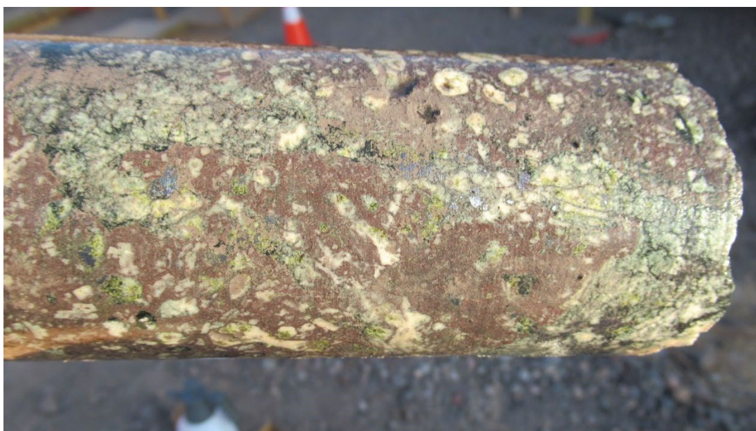
Figure 5: Altered Andesitic basalt ( MODD002 ) with fine grained disseminated pyrite, copper sulphides - chalcopyrite and bornite, and bornite amygdale fill
